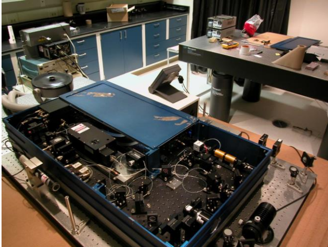
2 \mu m Doppler lidar transceiver provided by Earth Science Office (ESO) NASA Marshall Space Flight Center (MSFC)
