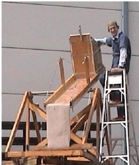
Figure 1 Water slide used to simulate lidar returns from river surfaces
