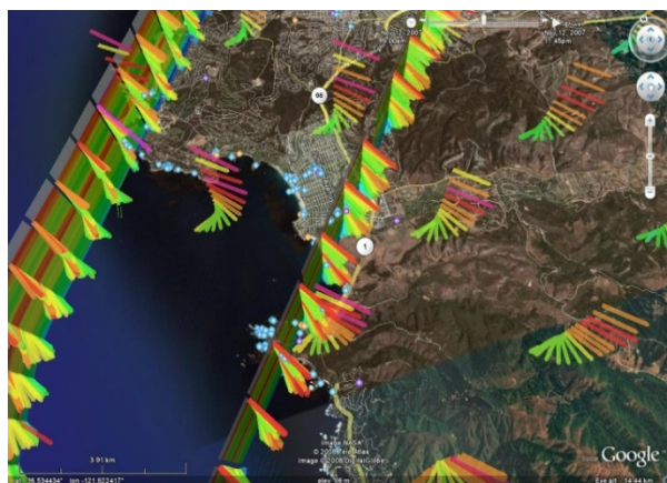
Figure 9 – Juxtaposition DWL wind cross sections with 4km MM5 meso-scale model output for same time period. The MM5 does not resolve low-level wind shear associated with fine scale flow about the local terrain.
