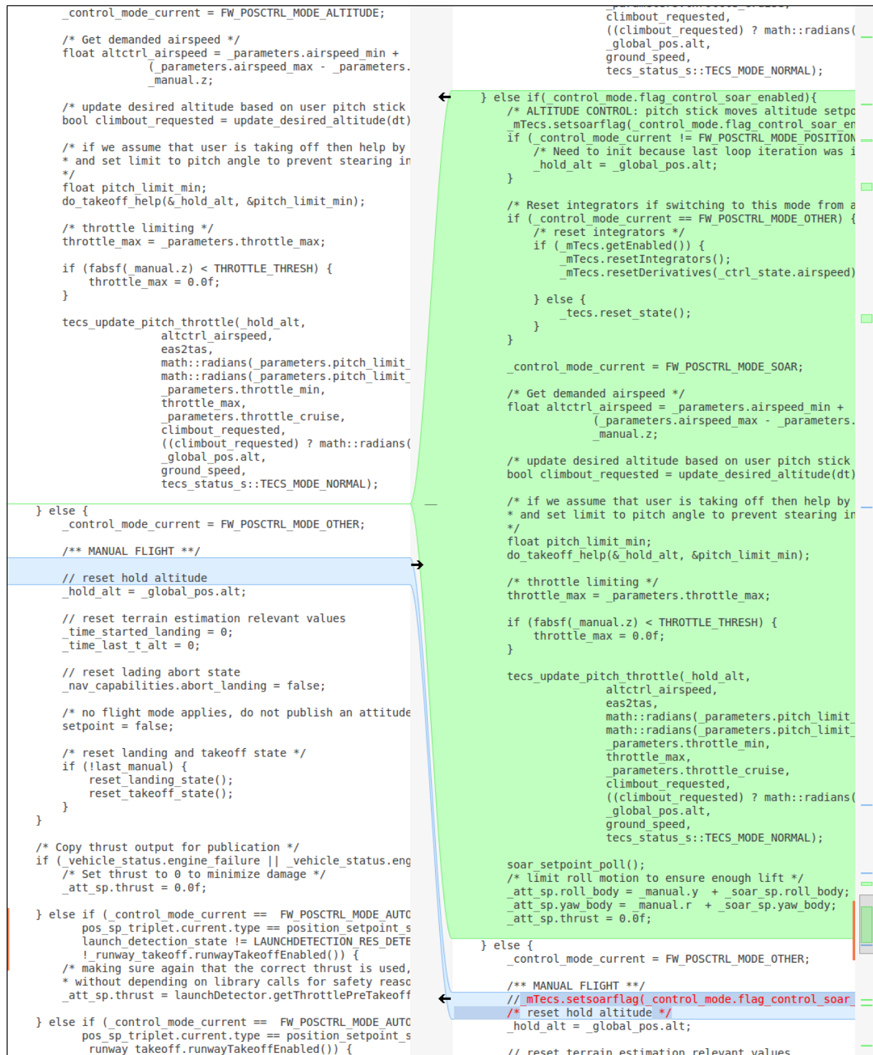
Figure 3: Version control software history showing addition of “soaring mode” to the attitude control module
