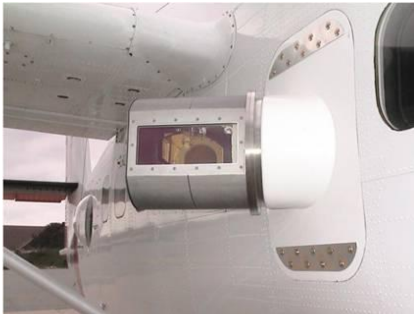
Figure 2.0 TODWL two axis scanner in Twin Otter side door.
